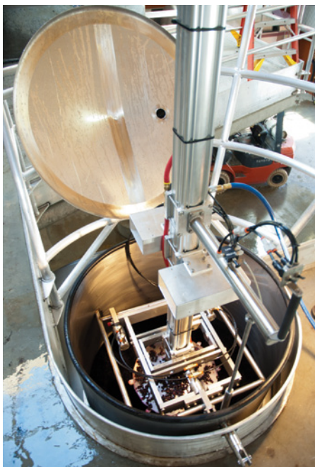
A portable pneumatic punchdown device attaches to bars on the upper manway turret, keeping the gimbal from rising while the foot of the device presses down on the cap.
