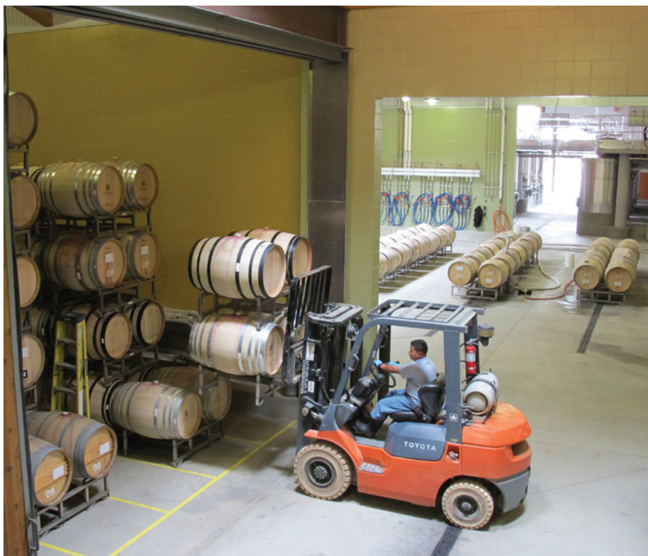
Easy removal of barrels from storage cell (left) to indoor barrel working area (left, background). Two reels drop nitrogen hoses from the ceiling (right) to provide nitrogen for a Racketeer debarreling wand, keeping the floor free of hose congestion for unencumbered activity.
