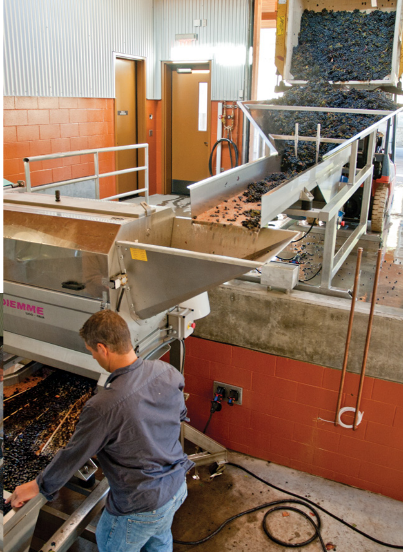
Receiving hopper and vibrating conveyor can deliver 8 to 10 tons/hour of grape clusters to the Kappa 25 destemmer (right). Grapes are sorted at 2 to 3 tons per hour, and fed to the pod for transport to fermentor (left).
