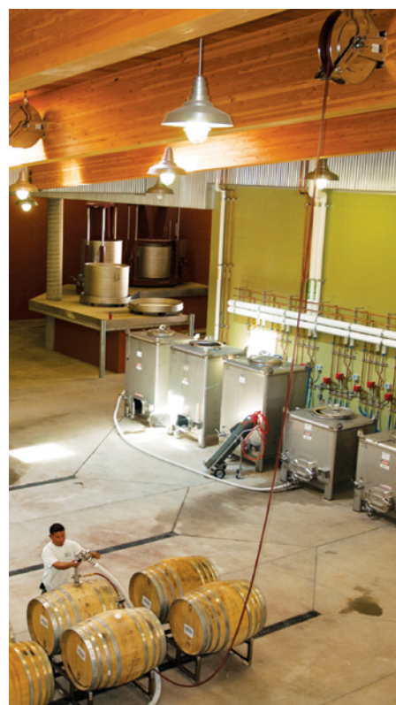
Easy removal of barrels from storage cell (left) to indoor barrel working area (left, background). Two reels drop nitrogen hoses from the ceiling (right) to provide nitrogen for a Racketeer debarreling wand, keeping the floor free of hose congestion for unencumbered activity.
