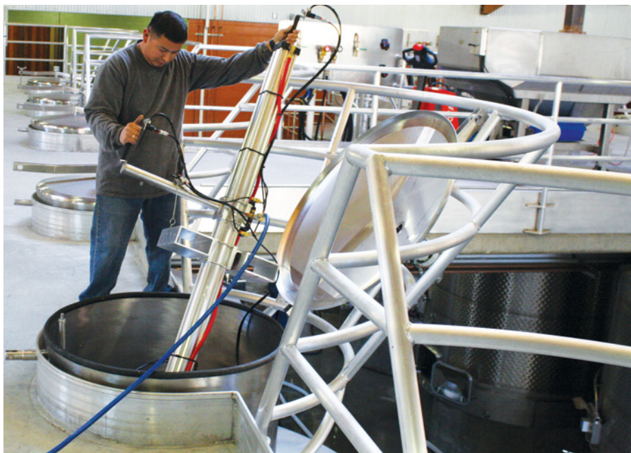
A portable pneumatic punchdown device attaches to bars on the upper manway turret, keeping the gimbal from rising while the foot of the device presses down on the cap.
