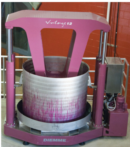
Halter Ranch has two Diemme "Vintage 12" basket presses for small red grape lots requiring careful pressing.
