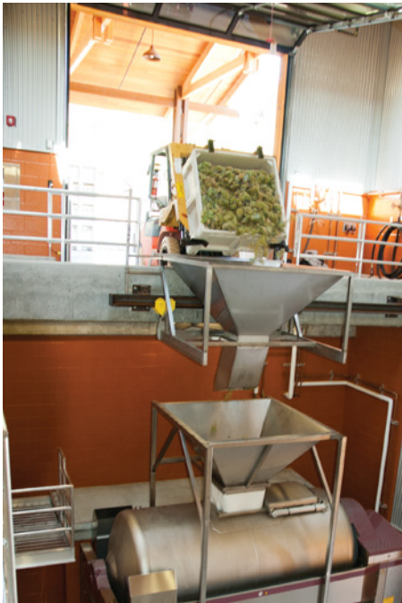
Dumping white whole clusters through the hopper into Diemme Velvet membrane press.
